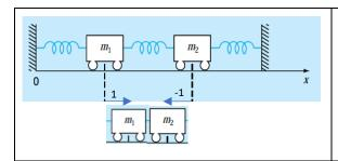
Unscaled eigenvector for mode #2 at  $\omega_2 = \sqrt{15}$
